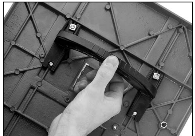
Figure 11. Sliding the trunnion onto the table.
